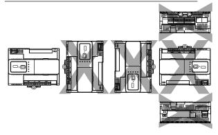
Installing the Device on a DIN Rail
