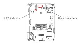
\*Note that the  $CO_2$  sensor has an optical bench that flashes. This is not the LED. The LED is at position D6 on the board. See diagram above.
