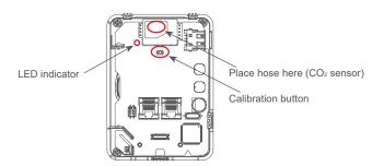
2. Start flowing nitrogen gas (0 ppm CO<sub>2</sub>). Use a flow rate of 0.3 to 0.5 liters/minute.
