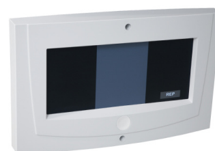
REP Sense Protocol Repeater duplicates the info serial communication line.
